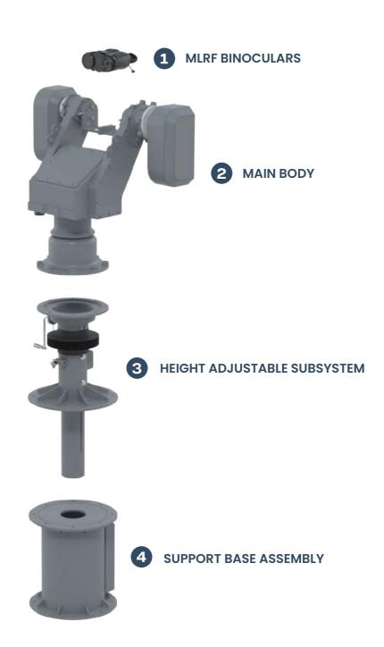
Figure above shows an exploded view of the Apollo TDS where it can be seen that the system is composed of 4 different
